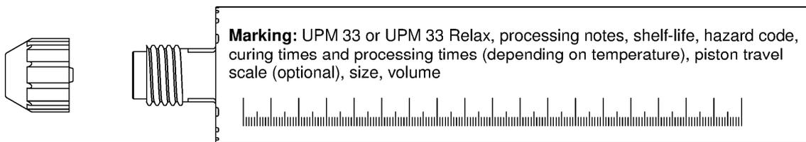
**Static mixer Upat MR Plus for injection cartridges from 300 ml to 410 ml**
