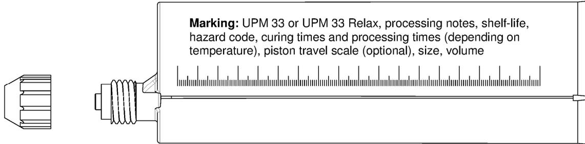
**Injection cartridge (coaxial cartridge) UPM 33 with sealing cap**
