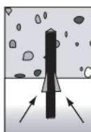
When installing overhead, clamp the anchoring element during the mortar hardening time using clamping wedges.
